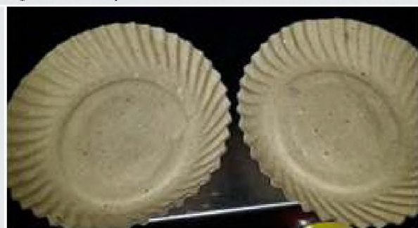
Fig. 3. Bee wax (emulsion) coated biomass-based plates showing hydrophobicity
