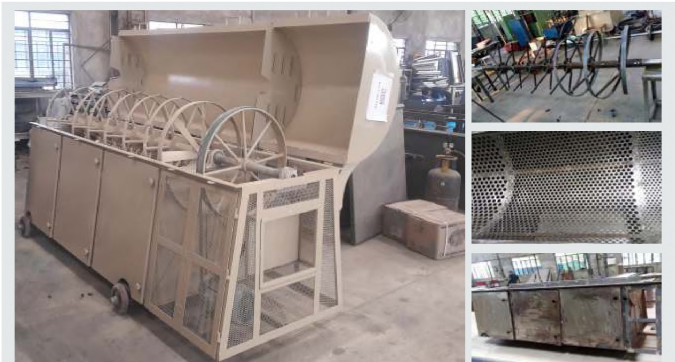
Fabrication of Boll Opener for processing of Kawadi Cotton in ginneries
