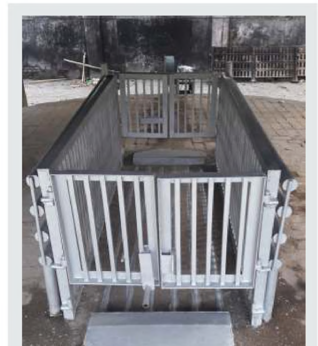
Modified ICAR-CIRCOT briquette-based crematorium installed at Ambazari Ghat, NMC, Nagpur
