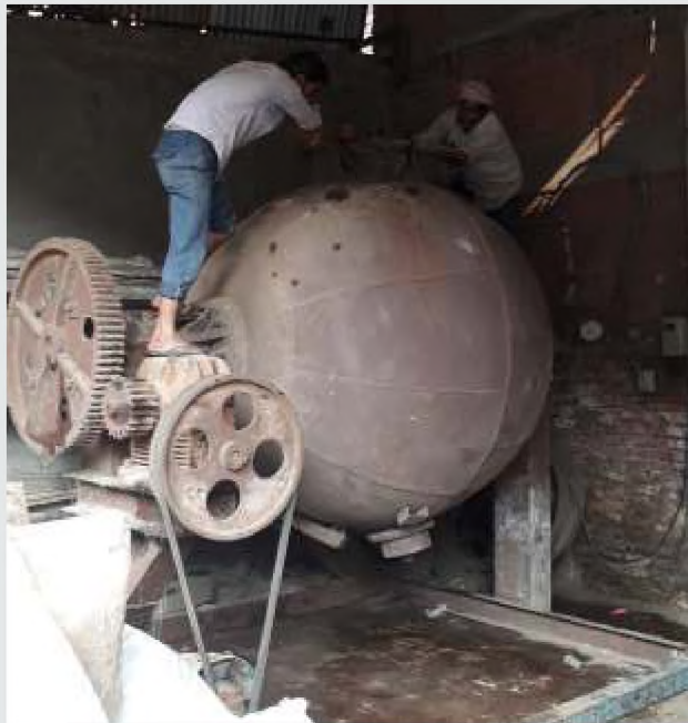
Industrial Pulping of Banana Fibres
