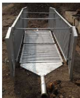
Experimental setup for burning of dead bodies using cotton stalk briquettes
