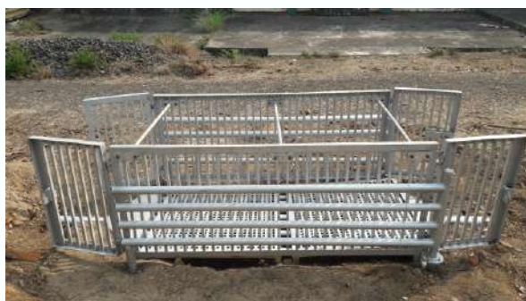
Experimental setup for burning of dead bodies using cotton stalk briquettes
