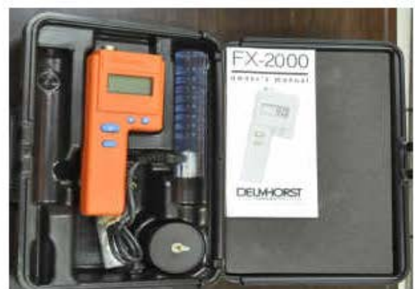
Digital Moisture Meter for measuring moisture in heaped biomass
