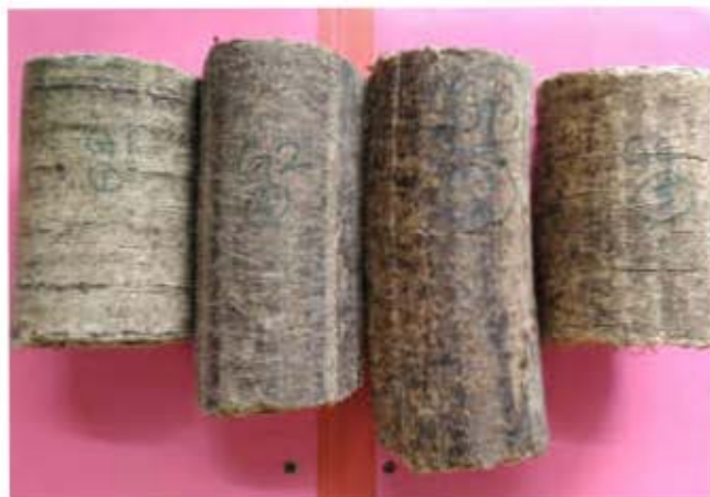
Fig. 2.11 Briquettes prepared from cotton stalks with 10% moisture content
