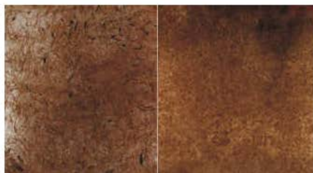
Fig. 2.14 Epoxy composite sheets from control and fibrillated samples
