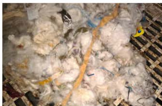
Fig. 2.4 Contaminants in Indian cotton (polypropylene, cloth bits, etc.)
