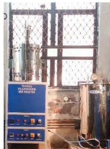
Fluidized Bed Reactor with Steam Generator
