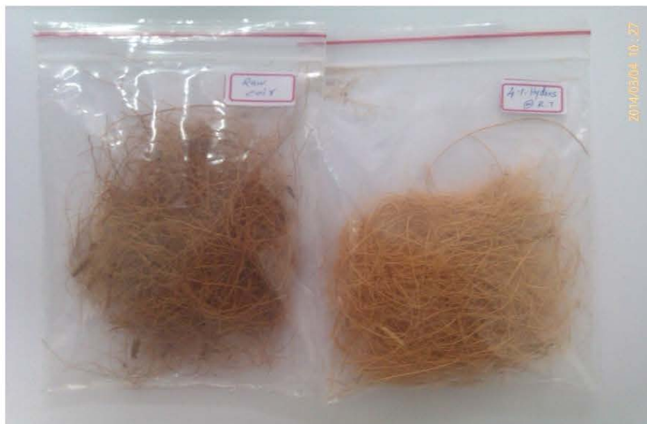
Fig. 13: Comparison of Raw Coconut Fibre and 4% \text{Na}_2\text{S}_2\text{O}_4 Treated at room temp.
