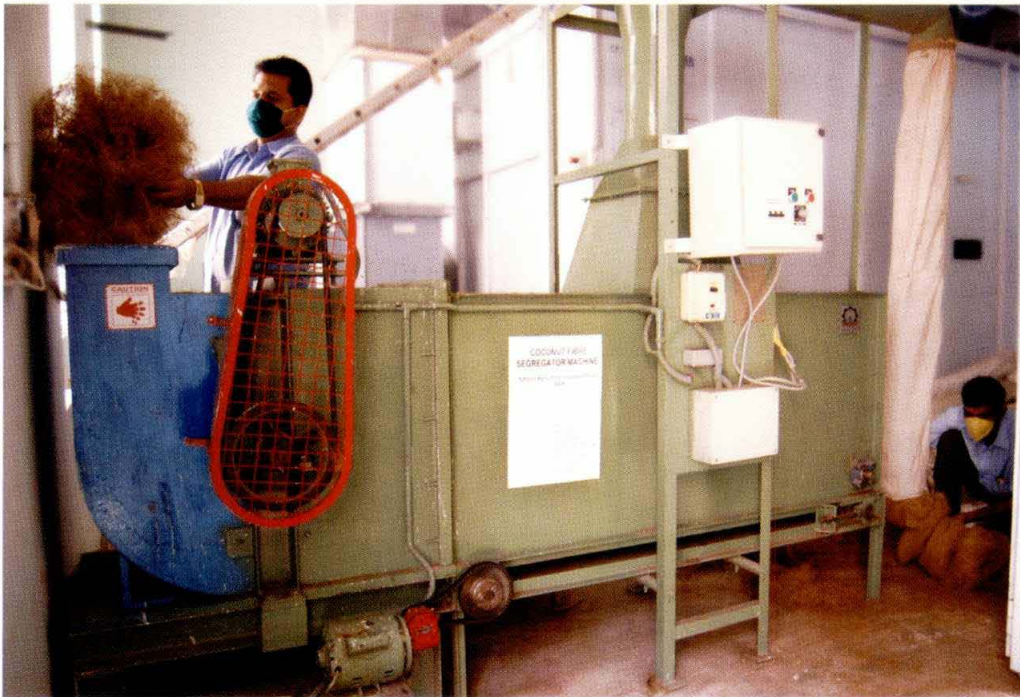
Fig. 5. Coconut Fibre Seggregator Machine Developed by CIRCOT
