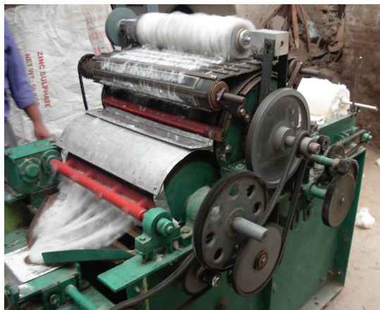
CIRCOT's sliver making machine
