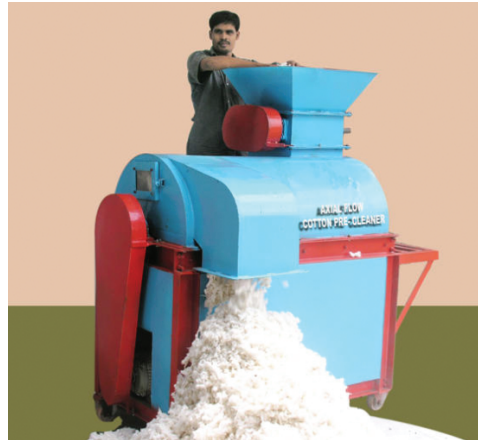
CIRCOT developed Axial-flow pre-cleaner
