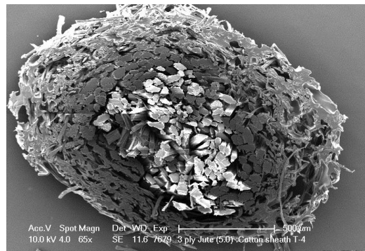
SEM of cotton covered jute
