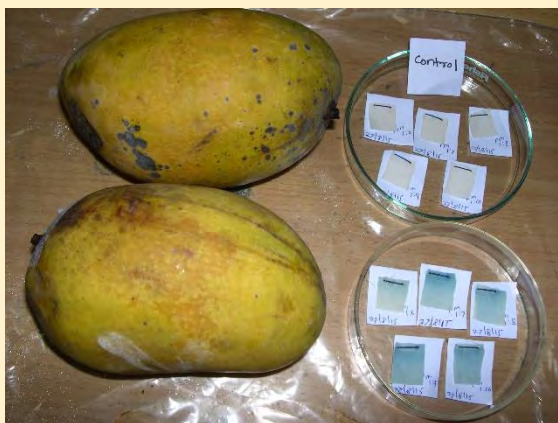
Electro spun fibre mat as sensor to monitor ripening of mango
