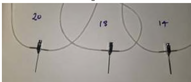
Fig 1b. Different Gauge multi-feed needle arrangement
