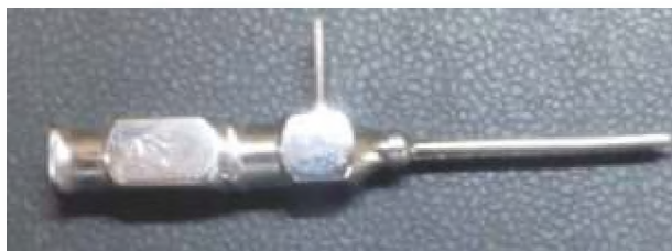
Fig: 1a Multi-feed electrospinning needle arrangements
