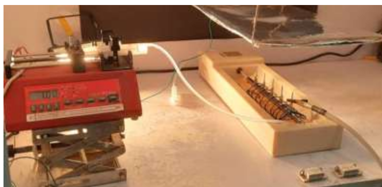
Fig. 12 Prototype of a spinneret arrangement with five nozzles
