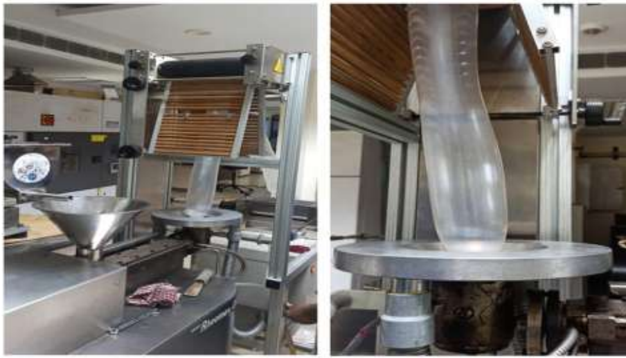
Fig.14 Blown film extrusion of the developed pellets
