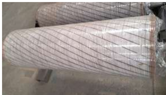
Fig. 6: Chrome Leather Roller of 381mm Diameter
