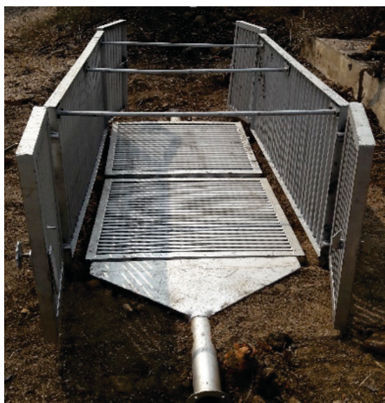
Experimental set up for burning dead bodies using cotton stalk briquettes
