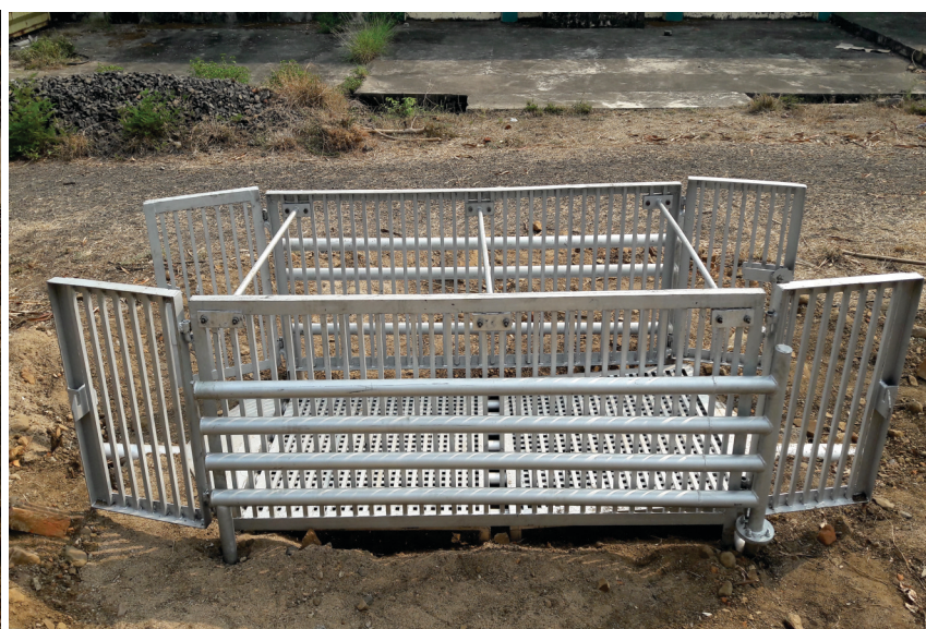
Experimental set up for burning dead bodies using cotton stalk briquettes
