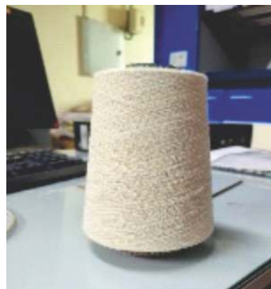
Fig. 2.6.4 Cotton blended banana fiber yarn
