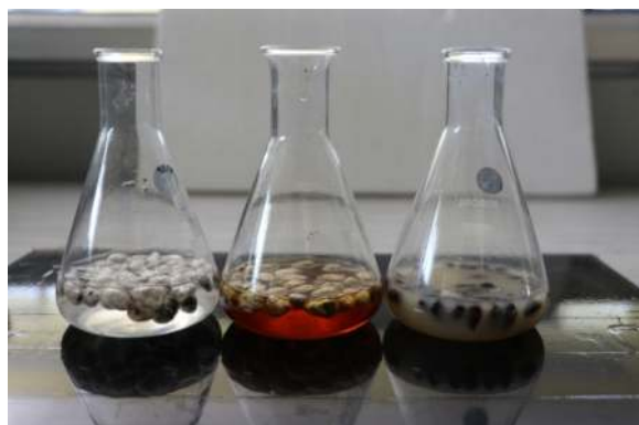
Fig. 2.4.2 Enzyme-mediated delinting process for cotton seeds and incubated at 50 °C in shaking water bath
