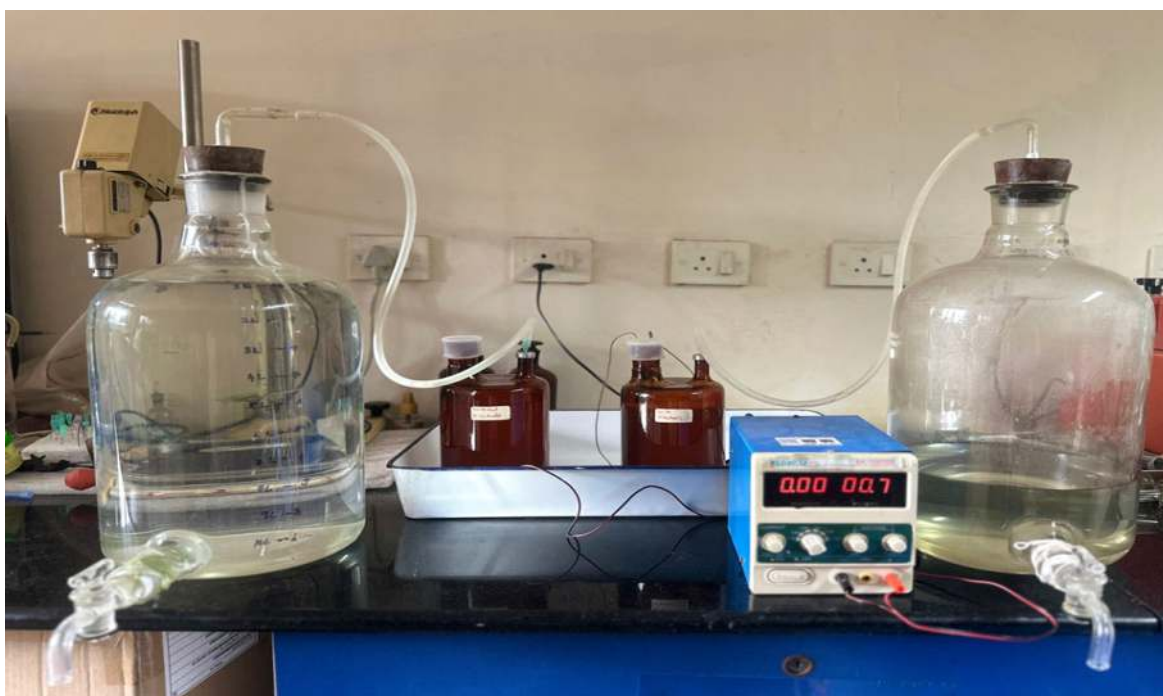
Fig 2.4.6. Microbial Electrolysis Cell (MEC) setup featuring amber reactors with graphite electrodes (powered by a DC supply) and aspirator bottles for volumetric gas collection via water displacement.
