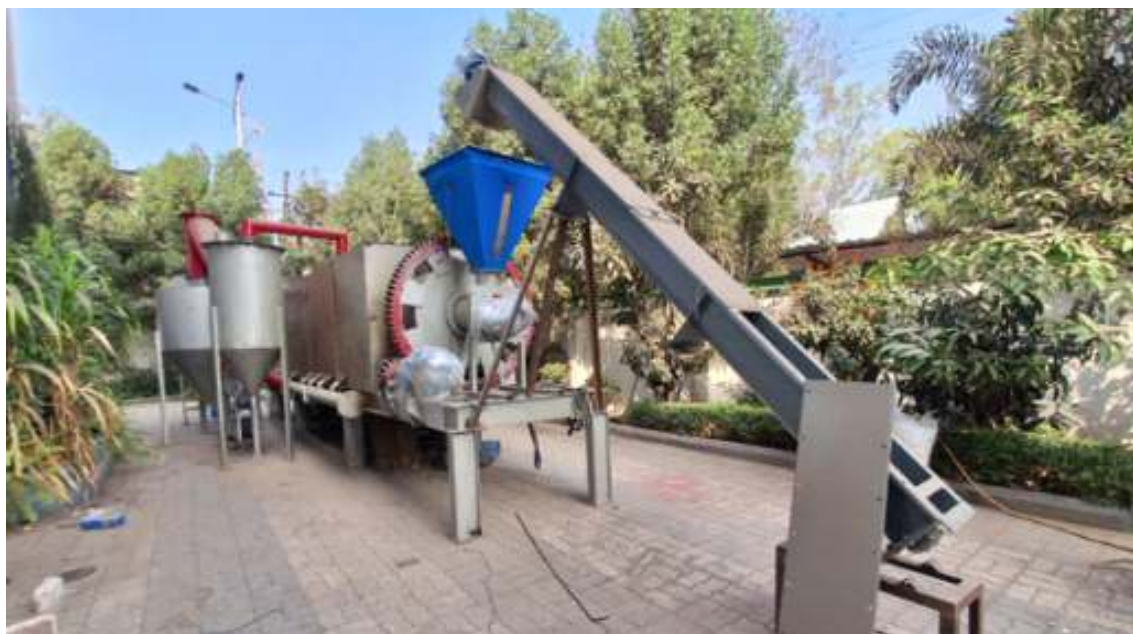
Fig.2.6.10 Fabricated pilot scale torrefaction unit (200 kg/h)
