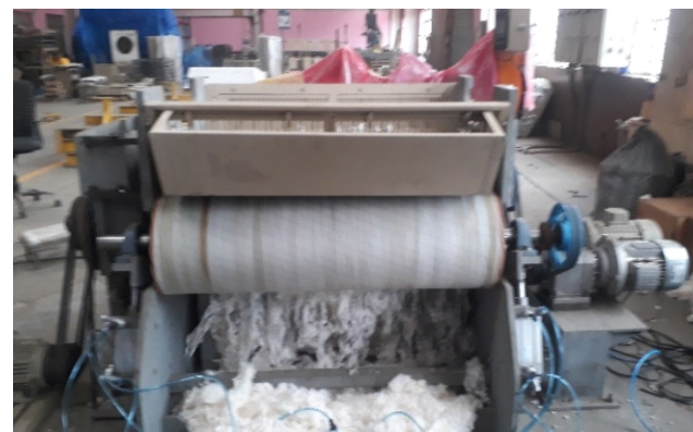
Fig. 1.5.2 HPDR gin with pneumatic type pressure mechanism
