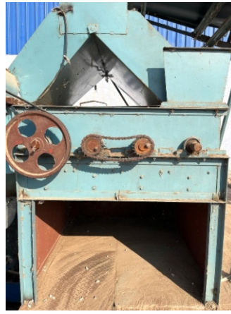
Fig. 1.4.2 Cleaning of pre-cleaner outlet
