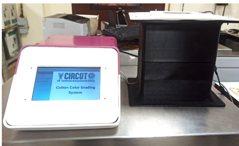
Fig. 3.4.1. Portable instrument to measure the colour grade of cotton
