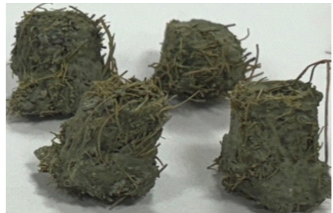
Fig. 2.8.2 Coir Composite cube after concrete after compression strength test
