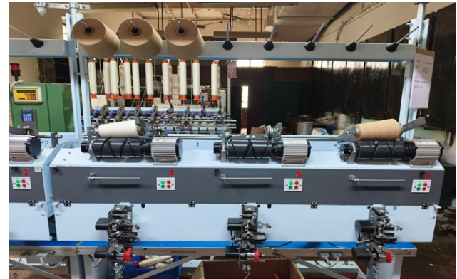
Cone Winding machine with EYC, splicing and fault classification
