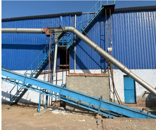
Fig. 1.4.1 Pneumatic conveying of seed cotton
