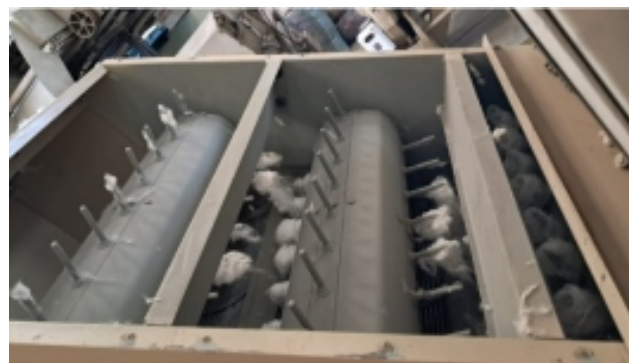
Fig. 1.1.2 Spade Type Cylinder Lint cleaner
