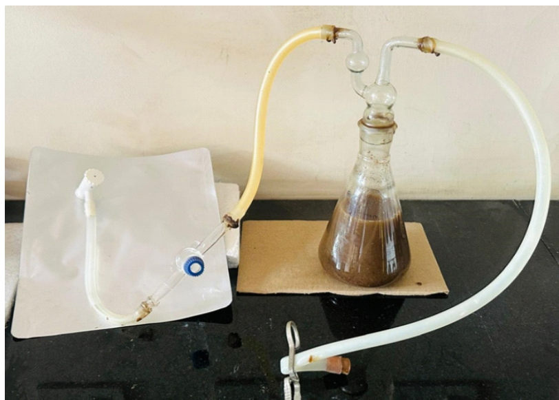
Fig. 4.6.1 Dark Fermentation setup for production of hydrogen gas
