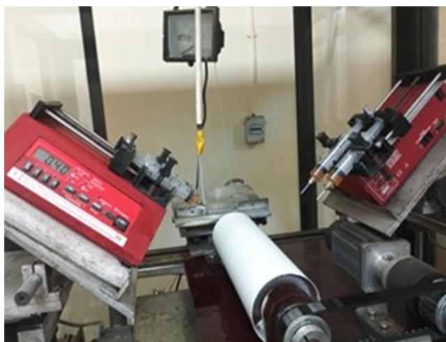
Fig. 2.1.1 Production of Multi-nutrient nanofibre sachet
