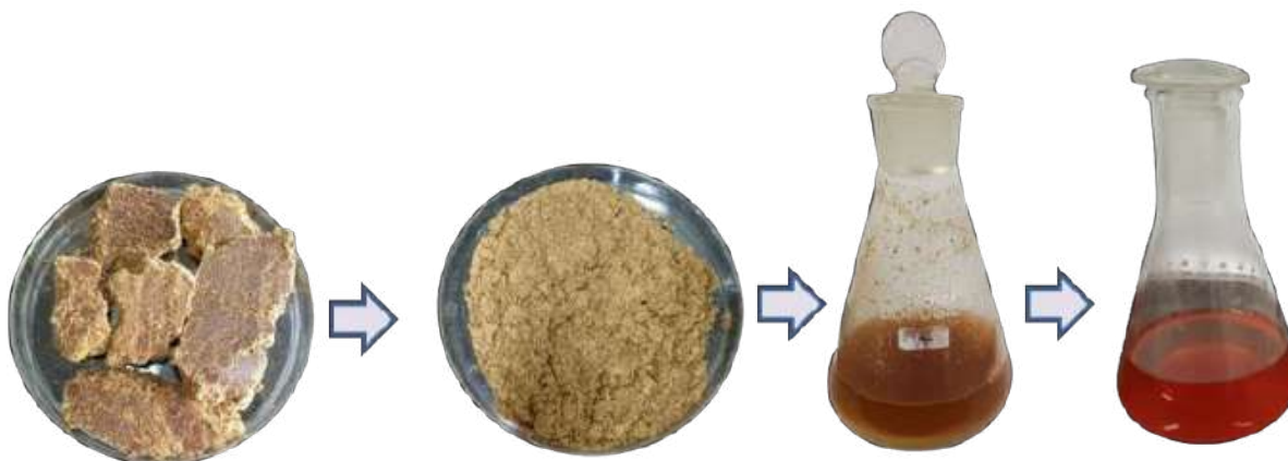
Fig. 2.19 Illustration of gossypol extraction from cottonseed meal 1
