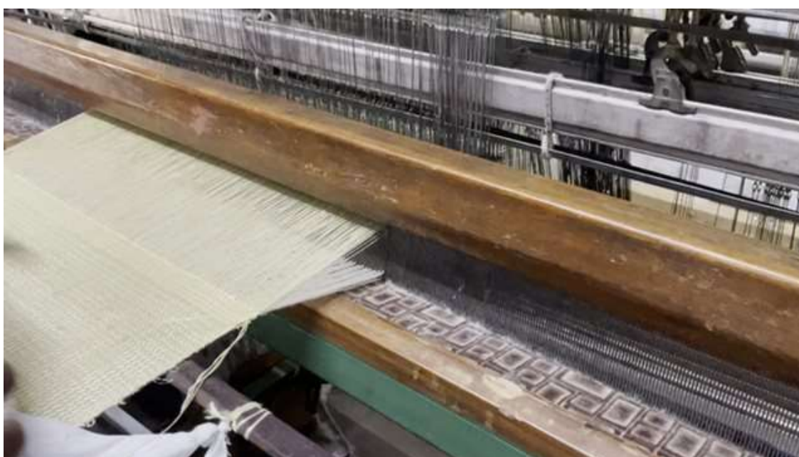
Fig 2.10 Multilayer Fabric weaving in a 2D weaving machine 1
