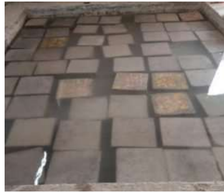
Curing of Concrete Cubes
