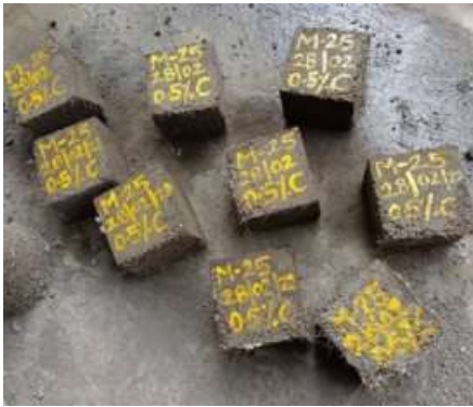
De-moulding of Concrete Cubes
