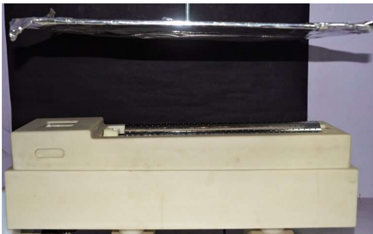
Fig: 2.5 Fabricated profiled rotating drum needleless electrospinning set-up 1
