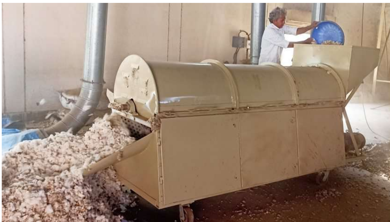
Fig. 2.11. ICAR-CIRCOT Boll Opener machine processing kawadi cotton
