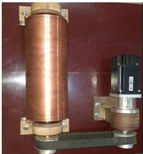
Fig: 2.36 (a) Fabricated rotating drum collector to produce aligned nanofibres (b) upgraded multi-phase electrospinning machine display (c) upgraded multi-phase electrospinning machine Panel
