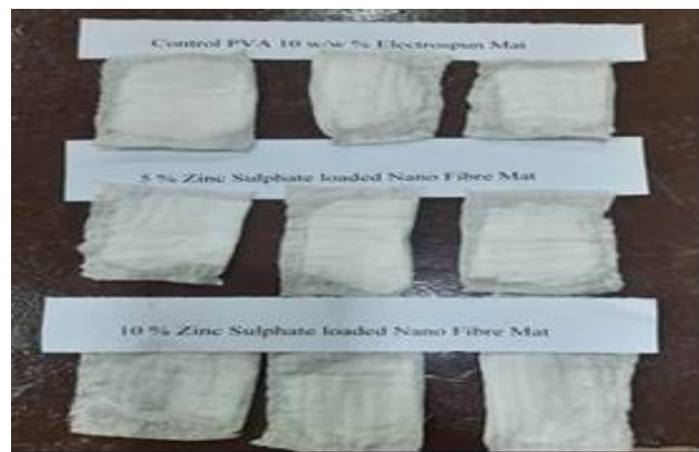
Fig. 2.13 Control, 5 wt% and 10 wt% Zinc Sulphate Micronutrient impregnated PVA electrospun Mat sachet for agriculture application
