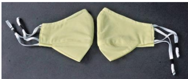
Fig: 2.34 Cotton based reusable face mask with breathability, antimicrobial and repellent property
