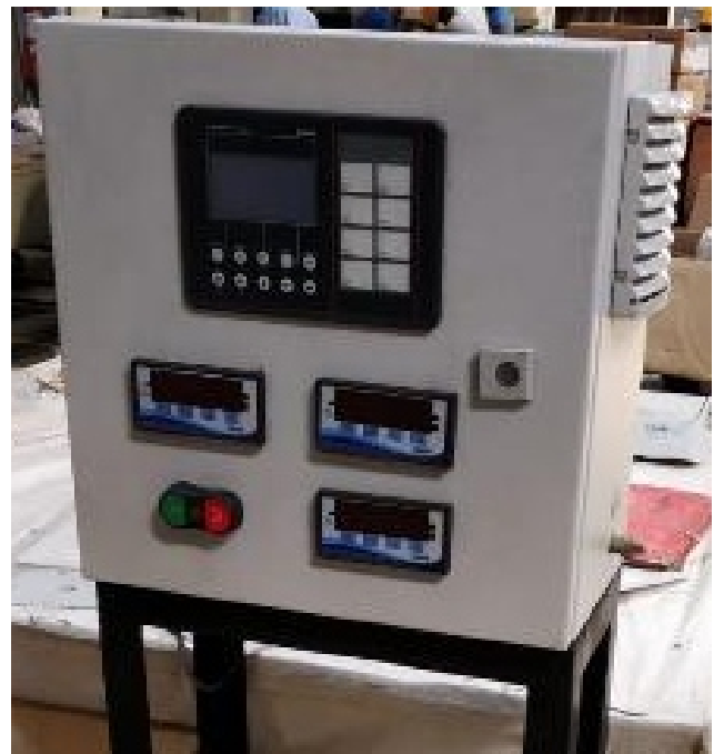
Fig. 2.1 GOC PLC setup with electronic display unit
