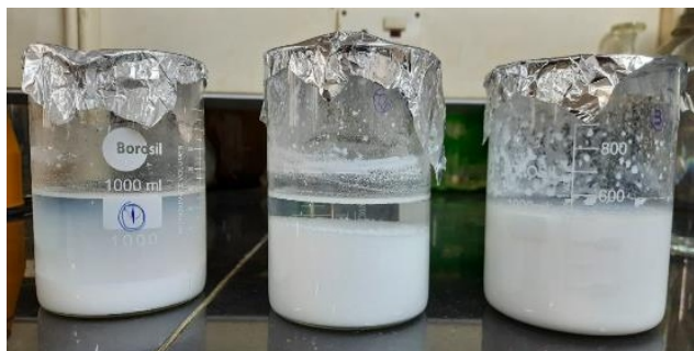
Fig. 2.23. Photograph of different nano-Zn formulations. Left one shows the nano-Zn stabilized by solubilized starch; middle one is without any stabilizer and right one is with CMC.
