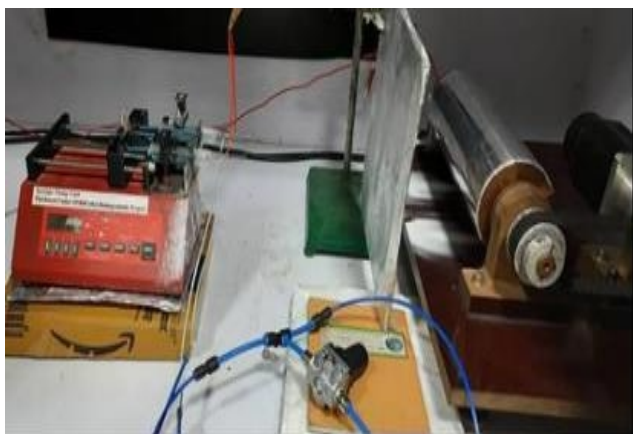
Fig. 2.14: Multi-feed High-pressure nozzle electrospinning setup
