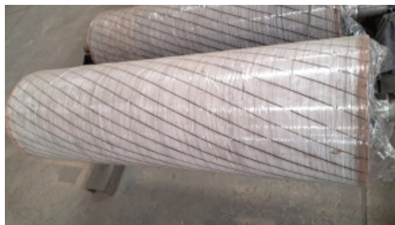
Fig. 6: Chrome Leather Roller of 381mm Diameter
