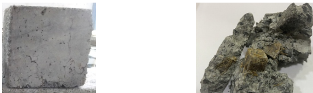
Fig.17 Coir fibre reinforced composite concrete cube before and after compression strength test
