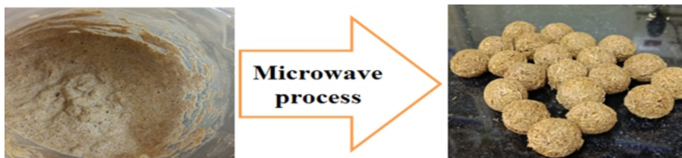
Fig. 19 Lignocellulosic foam from agro-residues
