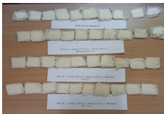
Fig. 13 PVA Electrospun mat with three multi-nutrients of different proportions
