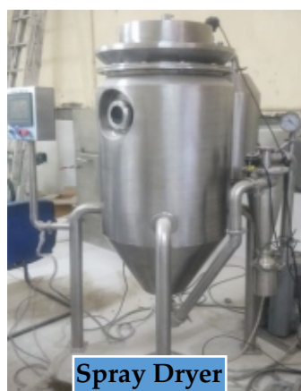
Fig 42. Pilot Plant for the extraction of protein from cottonseed
