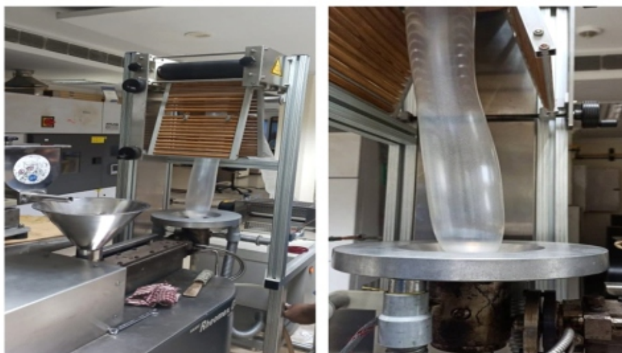
Fig.14 Blown film extrusion of the developed pellets
