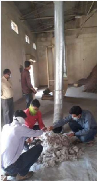
(a) Feeding of gin trash with PBW culture through inlet
