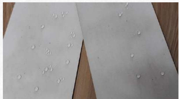
Figure 2. Hydrophobicity of sugarcane wax coated paper.
