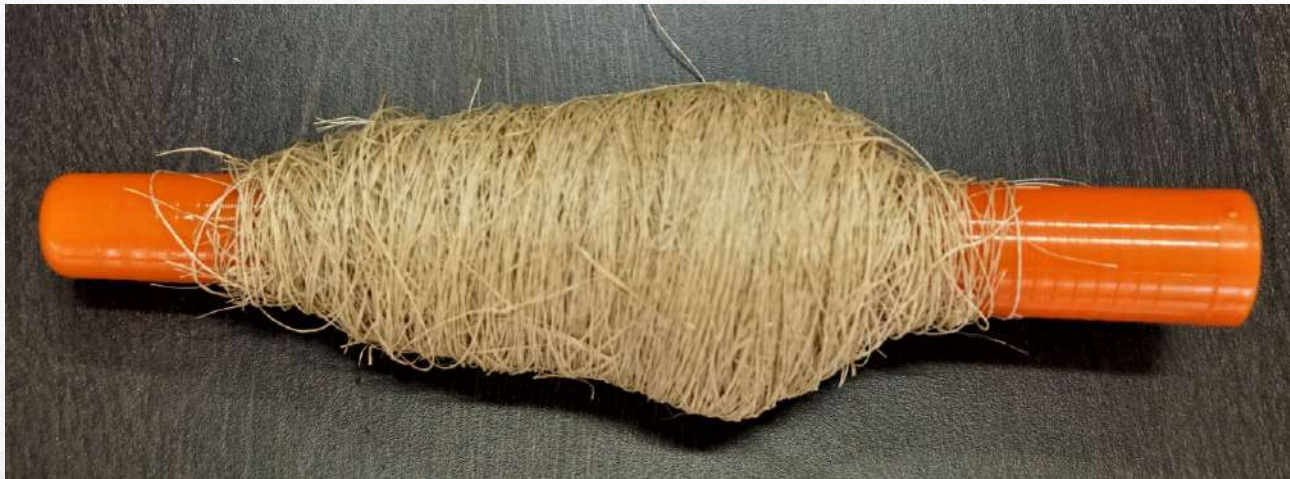
Figure 1. Banana fibre yarn developed at ICAR-CIRCOT
