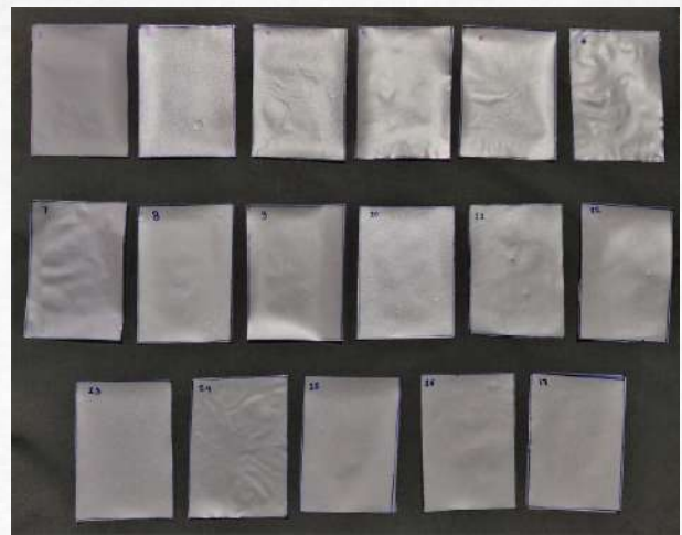
Figure 1: Nanocellulose reinforced starch based films prepared using 17 runs
