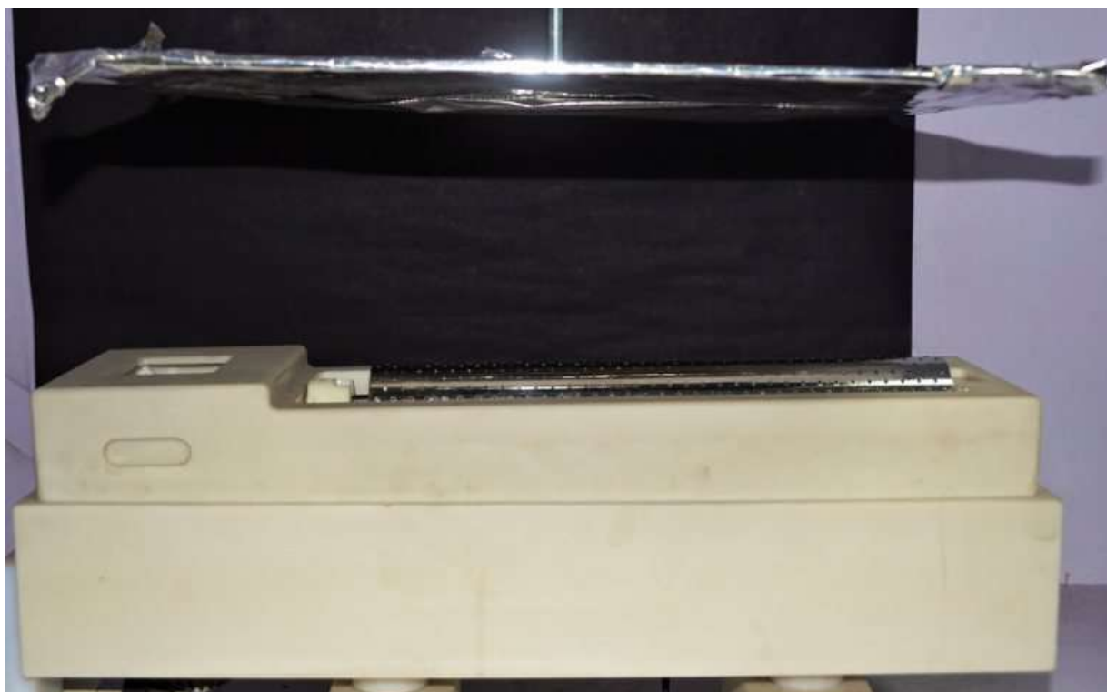
Fig: 2.5 Fabricated profiled rotating drum needleless electrospinning set-up
