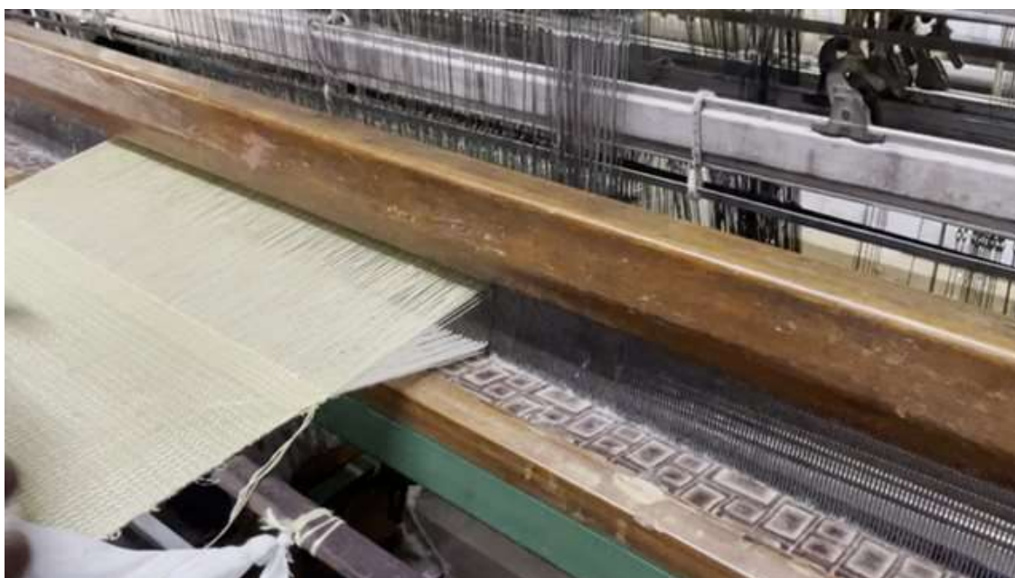
Fig 2.10 Multilayer Fabric weaving in a 2D weaving machine
