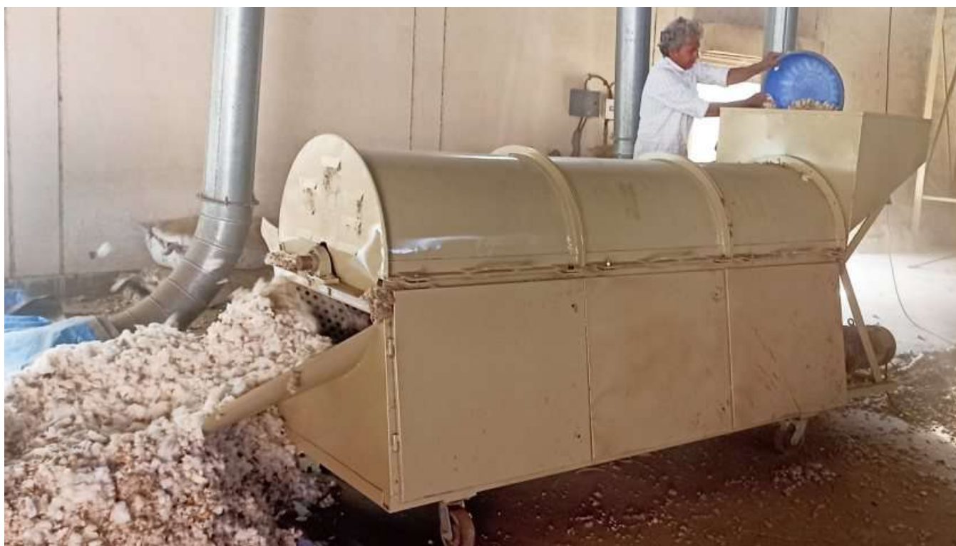
Fig. 2.11. ICAR-CIRCOT Boll Opener machine processing kawadi cotton
