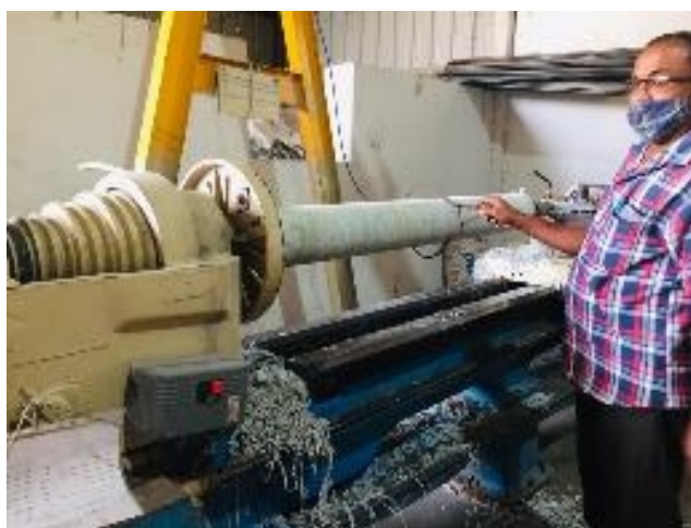
Fig. 2.5 (a & b) Modification of groove profile of chrome leather roller
