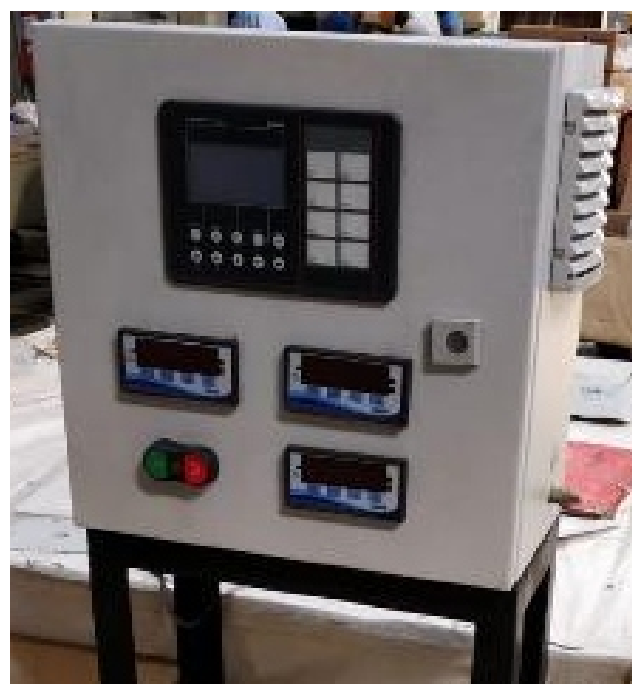
Fig. 2.1 GOC PLC setup with electronic display unit
