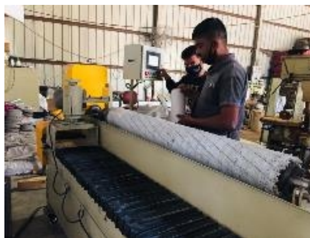
Fig. 2.5 (a & b) Modification of groove profile of chrome leather roller
