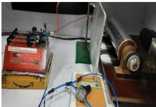
Fig. 2.14: Multi-feed High-pressure nozzle electrospinning setup
