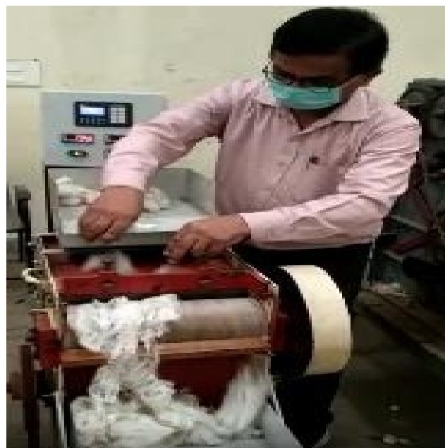
Fig. 2.2 Portable cotton gin with DGPI
