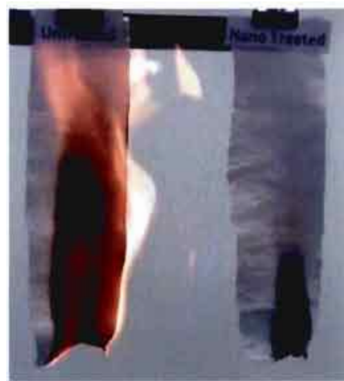
Fig. 2.16: Flame retardant cotton textile using nanoparticle (Left: Untreated and Right: Nano-treated)
