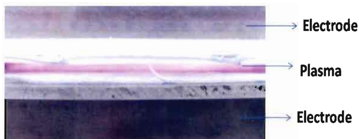
Fig. 2.21: Atmospheric pressure cold plasma generated in the mixture of helium-air gases
