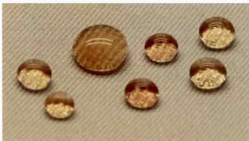
Fig. 2.15: Water droplets retained on cotton textiles indicating superhydrophobicity
