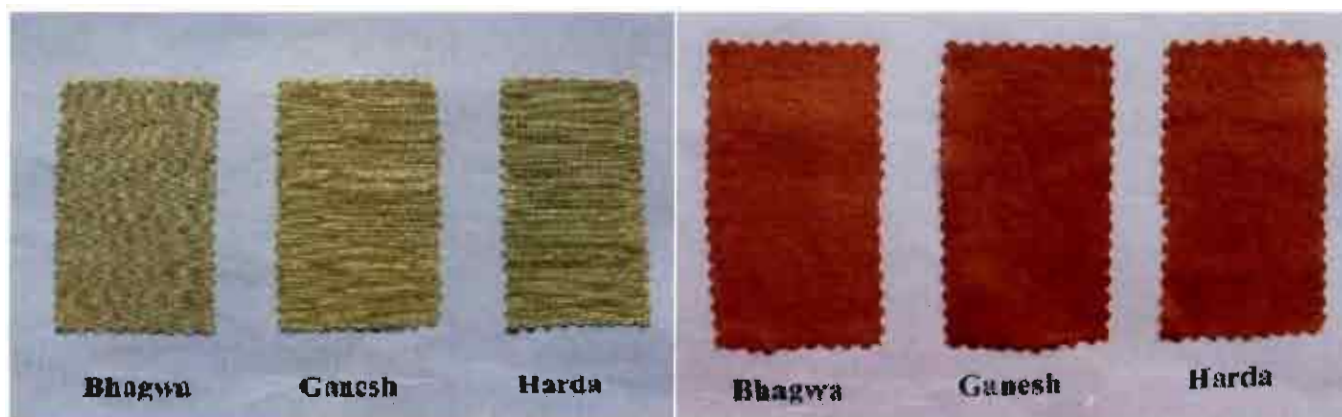
Fig. 2.18: Cotton fabrics mordanted with pomegranate rind powder and dyed to deep orange-red colour
